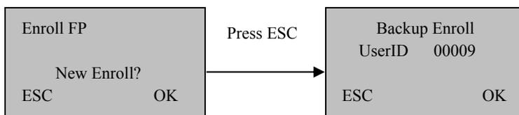
The backup enrollment steps are basically consistent with the new enrollment steps except that "Backup Enroll" instead of "New Enroll" is displayed on the top of the interface.
