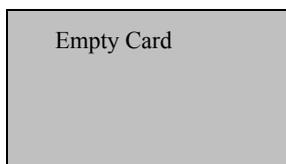
**Create PINCard:** This option is used to create an ID card for a user who has already been enrolled in the fingerprint lock. You can verify your ID card instead of your fingerprint (only after the parameter “Card Only” is set to “Yes”. For details, see 3.1).
