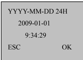
5) To modify date or time, press **▲/▼** to move the cursor to the desired option, and then press **▲/▼** again to enter correct date or time. Press **OK** to save your settings.
