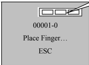
8) Press the same finger on the fingerprint sensor three consecutive times by adopting the proper finger placement mode. The system will prompt you to save the enrollment information after you enroll the fingerprint successfully. If enrollment fails, the system will prompt you to re-enroll your fingerprint.
