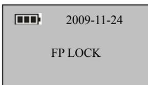
1) Power on the fingerprint lock by pressing the **Start** key to open up the initial interface, as shown in the figure on the left.
