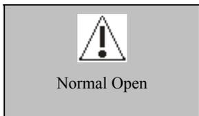
5) If you press **OK**, the interface as shown in the figure on the left will be displayed, indicating successful NO setting. In the meantime, the buzzer will beep three consecutive times.
