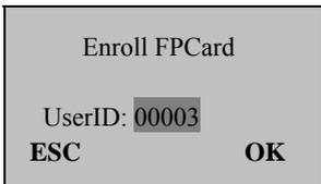
1) Select “User Manage” → “FPCard Mng” → “Enroll FPCard” from the main menu to display the interface as shown in the figure on the left:
