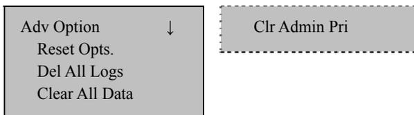
The options under “Adv Option” include: **Reset Opts.**, **Del All Logs**, **Clear All Data**, and **Clr Admin Pri**. Select any one of these options and press **OK** to display the related setting interface. Press **OK** according to the prompt to confirm your settings and return to the Adv Option interface, or press **ESC** to exit current interface without performing any operation.
