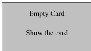
1) Select “User Manage” → “FPCard Mng” → “Empty Card” from the main menu to display the interface as shown in the figure on the left:
