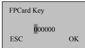
The FP card password consists of 6 digits. To enter a password, first select a digit from 0–9 by pressing **↑** or **↓** (You can press and hold **↑** or **↓** to rapidly scroll through the 10 digits) and press **OK** to confirm it. Then input the next digit in the same way until the last one. Finally, press **OK** to confirm the password and return to the System Opt. menu.
