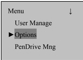
2) Press and hold the **Menu** key for three seconds to access the menu interface. Press **▼** to select “Options” and press **OK** to display the setting interface.
