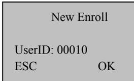
7) Enter the ID (ranging between 1 and 65534) to be enrolled behind the “UserID” option, and press **OK**, as shown in the figure on the left:
