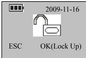
To disable the NO function, power on the system and press **OK** in the Normal Open interface. Then the system closes the lock and automatically powers off.
