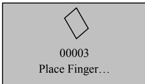
1) On the initial interface, swipe an enrolled FP card through the card reader. The interface as shown in the figure on the left is displayed:
