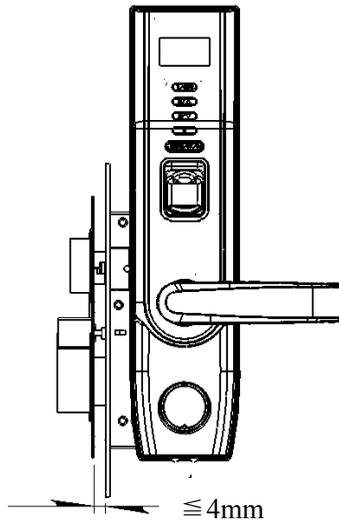
3. Please make sure of the door opening directions and lock body. Assume you are standing outside and facing a door and then there are four door opening directions: Left inward, left outward, right inward and right outward. Left inward/outward means the door swings inward/outward with hinges on the left; right inward/outward means the door swings inward/outward with hinges on the right, as shown in the following figure:
