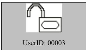
2) Place one of your fingers with fingerprint enrolled on the fingerprint sensor window properly. When the interface as shown in the figure on the left is displayed, the FP card passes the verification successfully.
