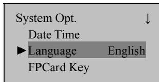
Press **OK** to display the Language interface, and press **▲/▼** to select a desired language. Press **OK** to confirm your settings and then press **ESC** to exit **System Opt.** When the system prompts whether to save your settings, press **OK** and your settings will take effect after system restart.
