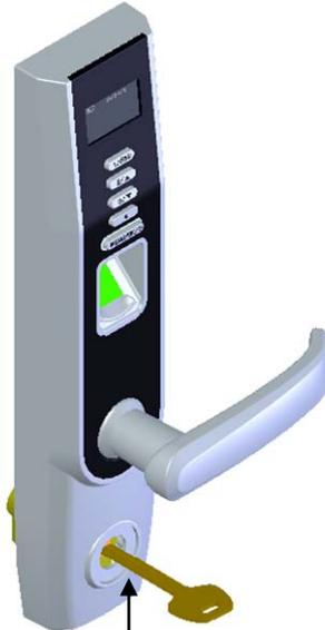
Insert the key into the keyhole and rotate 90°
