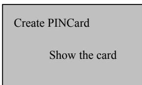
2) When prompted to enter the user ID number, press ▲/▼ to select the desired user ID, and press **OK**. The system then prompts you to “Show the card” (If the selected user ID does not exist in the system, the system will display a prompt “No Enroll”), as shown in the figure on the left:
